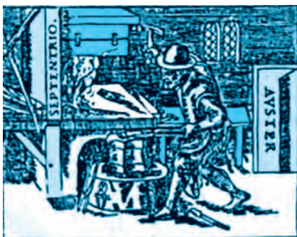
FIGURE 5.15 A blacksmith forging a permanent magnet by striking a red-hot rod of iron kept in the north-south direction with a hammer. The sketch is recreated from an illustration in De Magnete , a work published in 1600 and authored by William Gilbert, the court physician to Queen Elizabeth of England.
