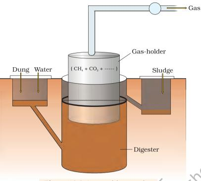
Figure 10.8 A typical biogas plant
