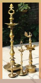
Nachiarkoil in Thanjavar District of **Tamil Nadu** is an important bell-metal centre. This is due to the presence of light brown sand called *vandal* on the banks of the Cauvery, ideally suited for making moulds. Some of the articles made by casting are vases in different shapes, tumblers, water-containers, plain and decorated ornamental spittoons which are a speciality of this place, foodcases, bells, candle-stands, kerosene lamps, picnic carriers, and a large variety of oil lamps.
