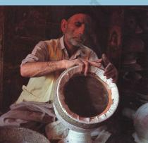
3. The surface is coated with a white layer of gypsum and glue and rubbed smooth with a stone or a piece of baked brick, called *Kurket*.
