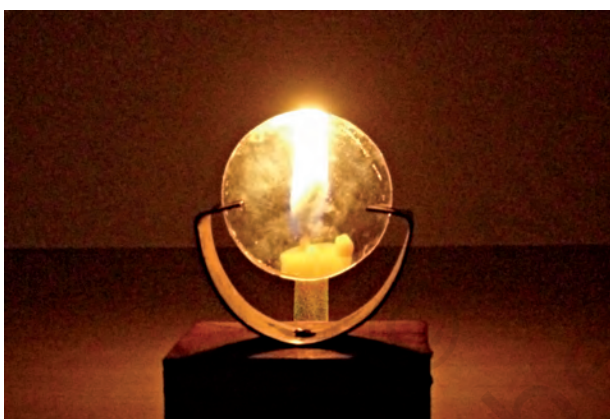
Fig. 15.26 Virtual image formed by the convex lens
