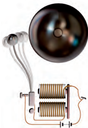
Fig. 14.20 Circuit of an electric bell
