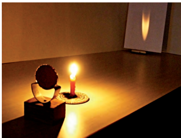
Fig. 15.15 Real images formed by a concave mirror
