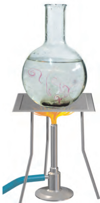
Fig. 4.9 Convection of heat in water
