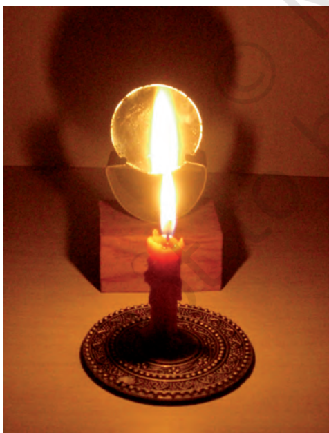
Fig. 15.16 Virtual image formed by a concave mirror
