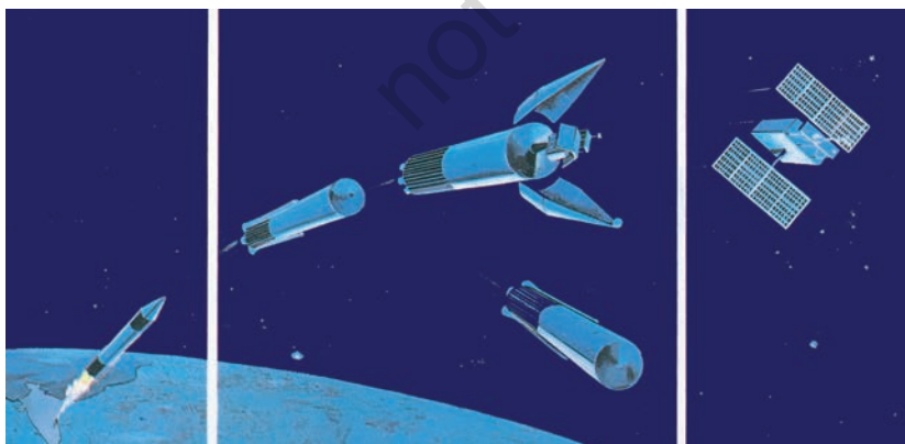
Rocket launch Rocket falls back to the Earth Satellite enters orbit Figure 1.4 : Human-made Satellite
