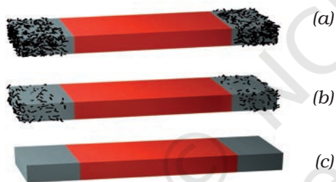
Fig. 13.6 Magnet with (a) many iron filings (b) few iron filings and (c) no iron filings sticking to it.
