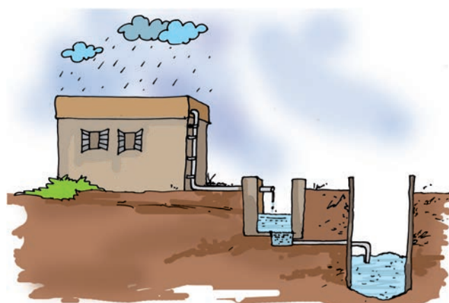
Fig. 14.13 Rooftop rainwater harvesting
