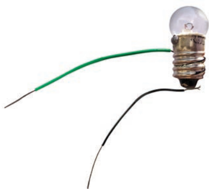
Fig.12.4 Bulb connected to two wires
