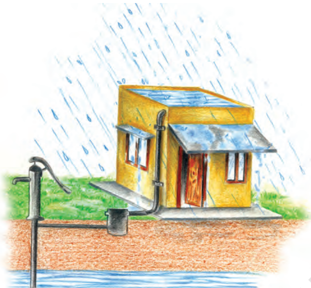
(a) Recharge through Hand Pump
